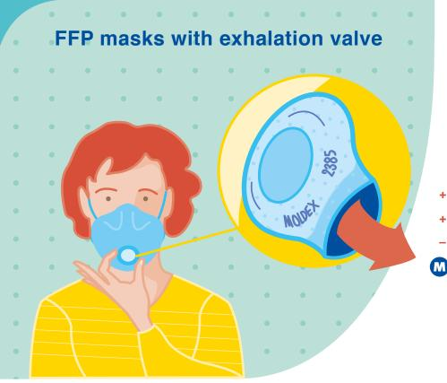
The valve on an FFP mask is an additional comfort feature. It opens when you breathe out and remains tightly closed when you breathe in. This way, warm and humid exhaled air is expelled from the mask. This ensures a more pleasant climate inside the FFP mask and exhalation is easier.
